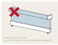
Automated screens are very easy to use, upper and lower limits are set during installation. On the remote simply push the button (up/down) to lower or raise your screen, this can be stopped in any position by pushing the centre button.
