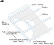
Use **Noise Stop Tape** on all battens, purlins or noggings to minimise the noises associated with expansion and contraction.
